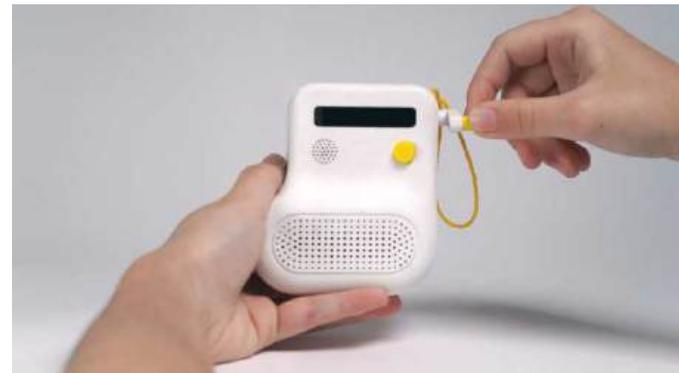
Considering **ergonomics**, I designed it to be **easy to hold**—a protruding curve on the left side facilitates gripping with the left hand, making users feel **stable and comfortable** when rotating the handle with the right hand.
